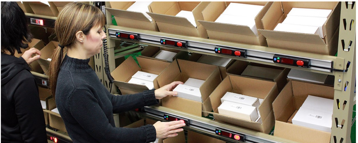
Obrázek 7 Pick by Light (Lightning Pick, 2023)
