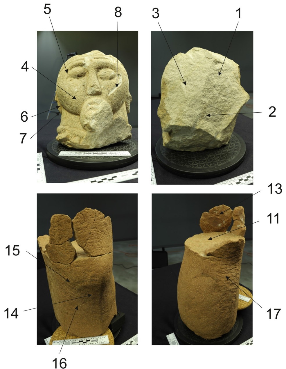
Fig 10. Points of the X-ray fluorescence measurements (author: M. Cihla and F. R. Václavík).
