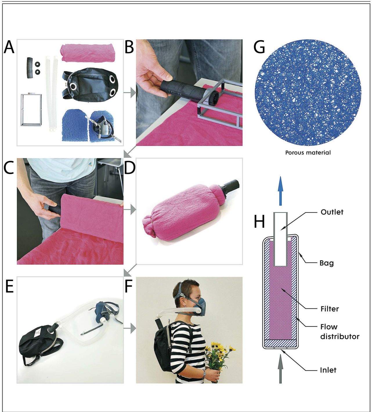
Fig 3. Assembly scheme of the filter kit. Shown are all parts of the filter kit (Panel A) and its gradual assembly (Panel B-E), including a demonstration of how it is to be worn (Panel F). The purpose of the blue porous material on Panel G is to allow air to access the filter cartridge; air is sucked in over its entire surface (flow distributor). On Panel H the cross-section of the filter kit and the direction of air movement are shown.
