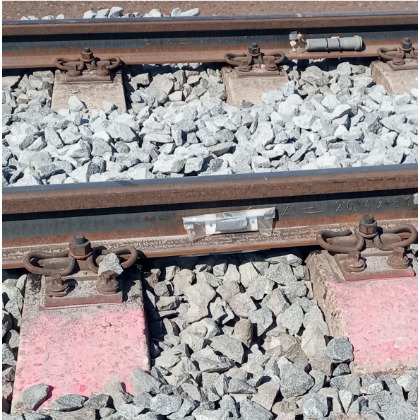
Figure 3.14 – Position of the Thermometer at the Left Side of the Rail Web in the Borovnice Locality
