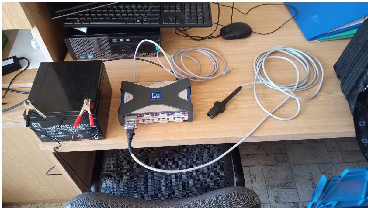
Figure 4.14 – Measuring Set Mobile Unit
