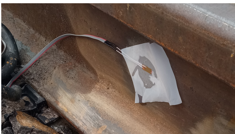
Figure 3: Strain gauge attachment by 1-70 fast-acting superglue.
