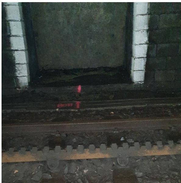
Figure 3.29 – Harrachov Locality – Position of a Thermometer in Polubenský Tunnel (Thermometer from the bottom of the Rail Foot), Author Dr. Vladimír Suchánek
