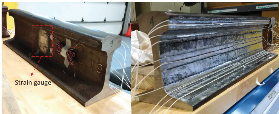
Figure 2.7 – Rail Specimen Instrumented with Strain Gauge and Optical Fibres [16]
