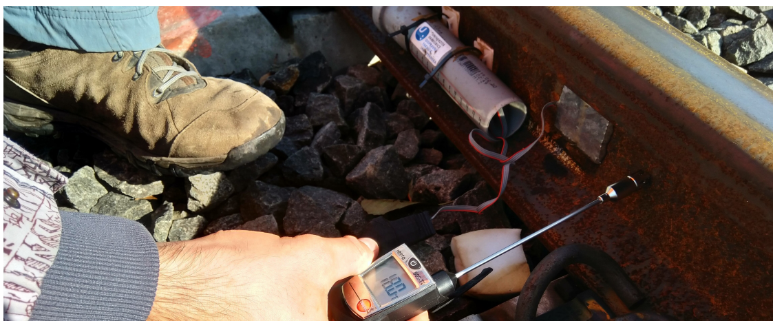
Figure 2 – Temperature Measurement by Surface Thermometer with Parallel Connection of Track and Mobile Unit of Measuring Set (in the Background).
