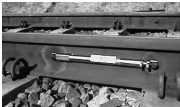
Figure 2.4 – MS-02 Extensometer for Measurement of the Longitudinal Forces in Rails [24]
