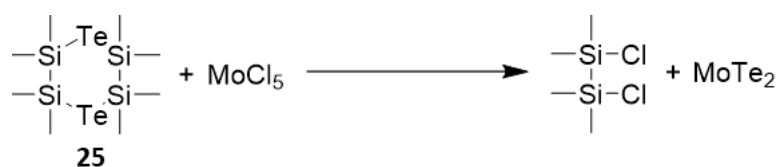
Scheme 10. Reaction of MoCl 5 with 25 resulting in MoTe 2 thin film.
