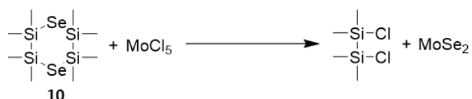
Scheme 7. Formation of MoSe 2 thin film by reaction of MoCl 5 with cyclic precursor 10 as an example.
