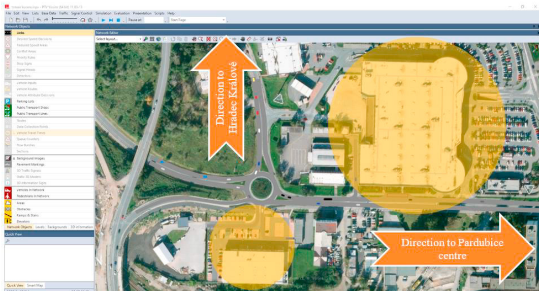
Fig. 4. Use of the PTV VSSIM software with modelled lines (roads) and insertion of vehicle inputs.
