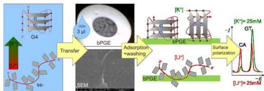
Fig 1. Scheme of the adsorptive transfer stripping voltammetry representing stabilization of guanine reach ODN sequence into the guanine quadruplex (G4) by \text{K}^+ in the solution, transfer of the ODN aliquot on the bPGE surface with representing SEM image (magnification 10.000x) and schematic arrangement of the folded G4 and unfolded single stranded (ss-) ODN adsorbed on bPGE together with following I - E curves representing differences in CA and GT peak currents in presence of 25mM \text{K}^+ or \text{Li}^+ in the solution from which ODN has been adsorbed.
