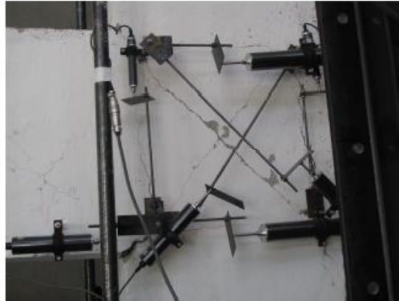
Fig. 2. Comer to comer cracks in X pattern.
