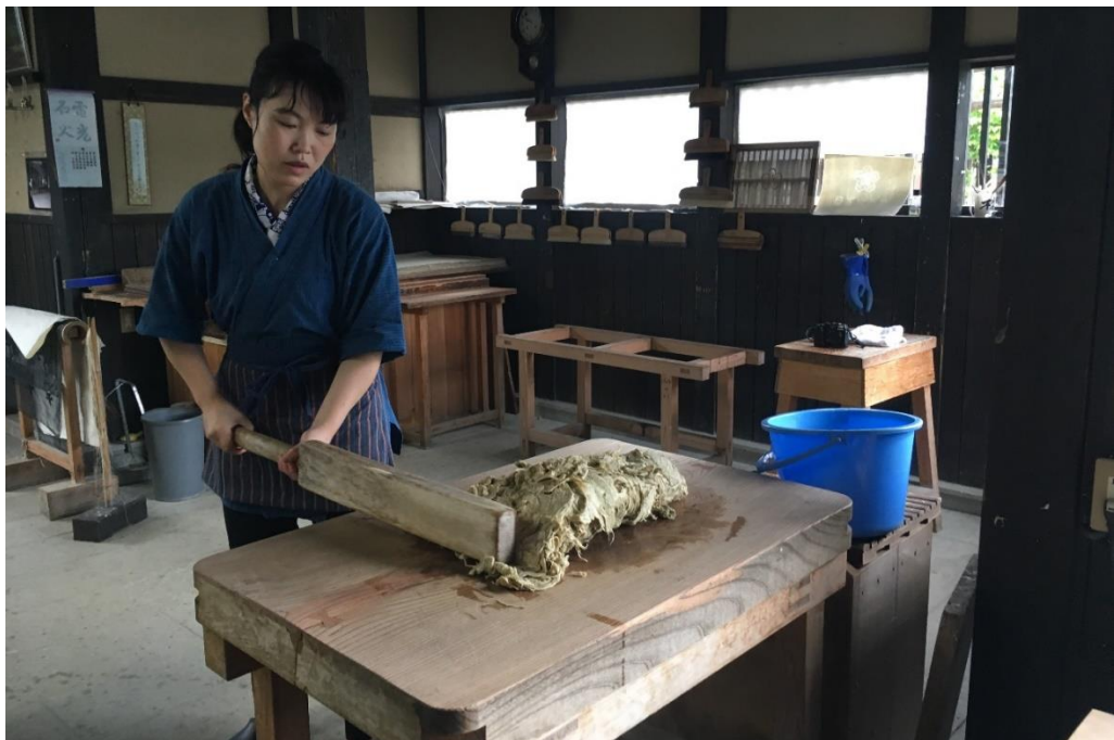
Figure 69. Japanese method of pounding the bast.
