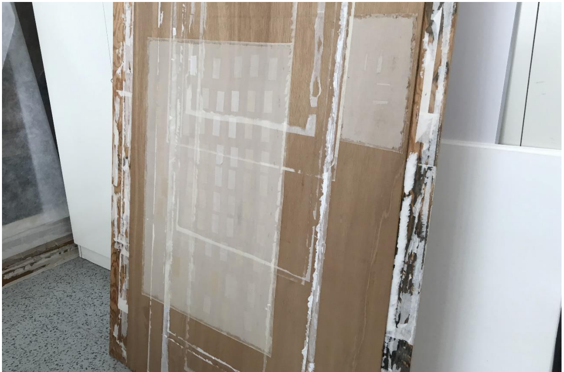
Figure 152. Process of the experiment, flattening the samples on a drying board.
