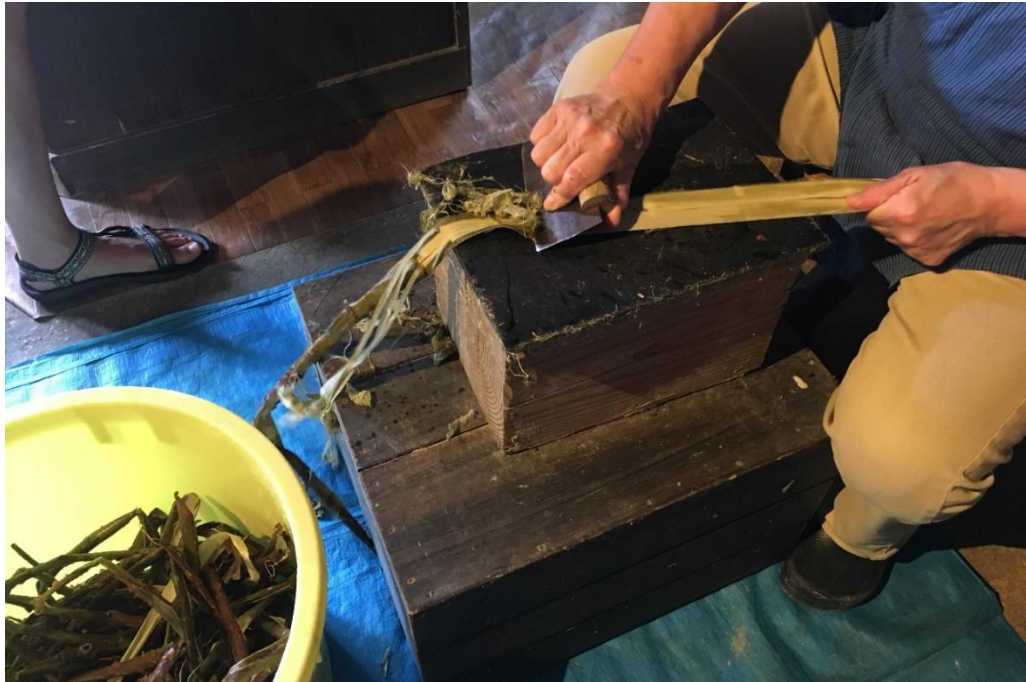
Figure 68. The process of separation of the green and brown parts of the bark from the white parts of the bast.
