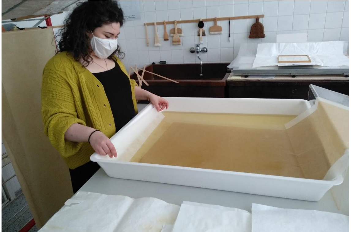
Figure 132. Preparation of the dye for toning paper from yasha cones, washing away residues of potash.
