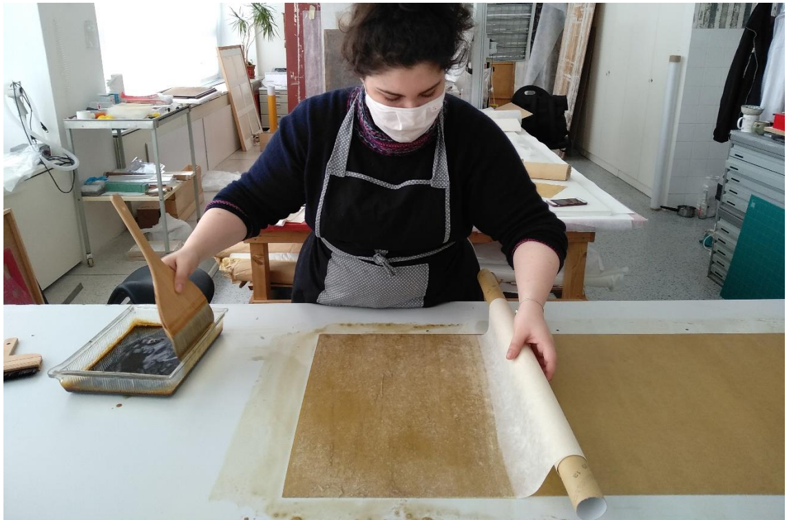
Figure 131. Preparation of the dye for toning paper from yasha cones, application of the dye using brush.
