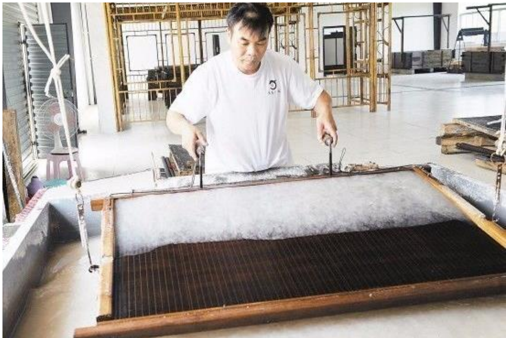
Figure 73. Process of forming sheets of paper using paper pulp, Chinese method. 62
