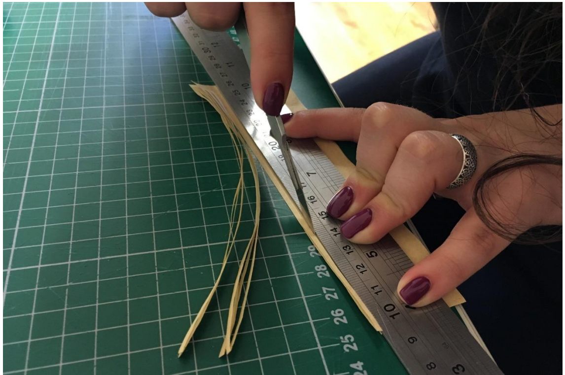
Figure 118. Preparation of reinforcement strips tiaozi , cutting process.
