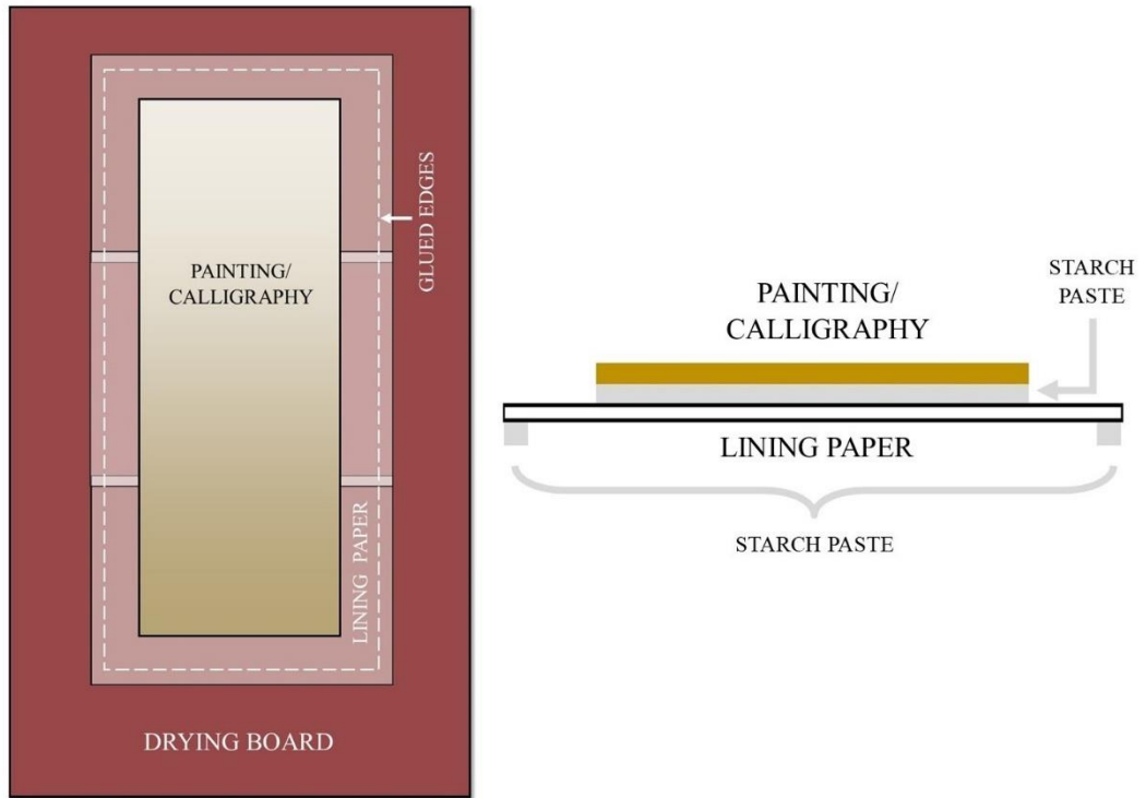
Figure 125. Scheme of application of an object to the drying board using the edges of the lining paper.
