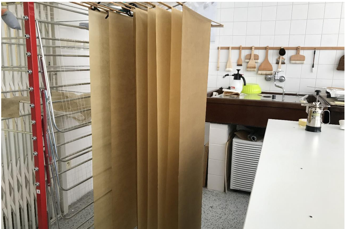
Figure 36. Process of the treatment, process of toning paper using dye from yasha cones, drying paper.
