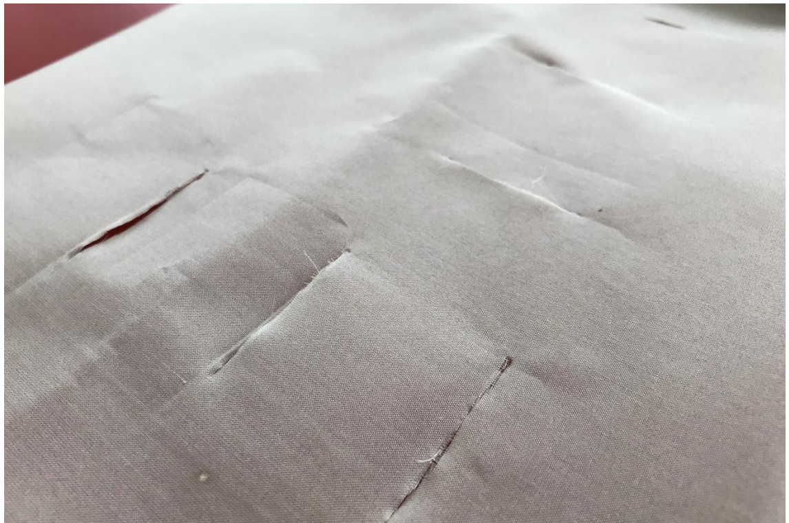
Figure 150. Preparing of the silk support for the experiment: The mechanical damage to sized silk.
