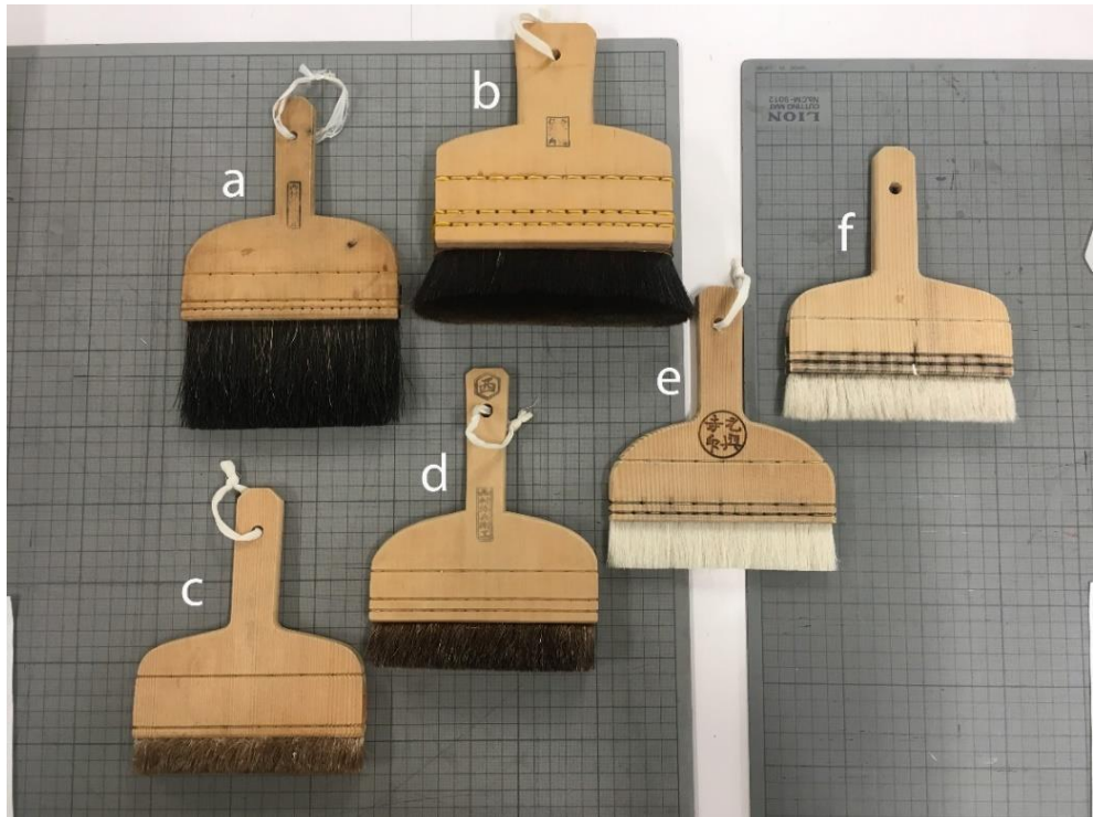
Figure 136. Japanese brushes with their Chinese equivalents: a) nadebake (Japanese) – smoothing brush, b) uchibake (Japanese) / tsung bi shua (Chinese) – tapping brush, c) d) mitsubake (Japanese) / shui shua (Chinese) – brush for water processes, e) noribake ( tsukemawashi-bake ) (Japanese) – brush for the application of glue, f) noribake (Japanese).
