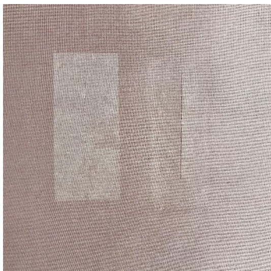
Figure 153. Surrogates with a tear along the weft direction mended with: a) paper patch; b) textile patch using adhesive Klucel G, dark background.
