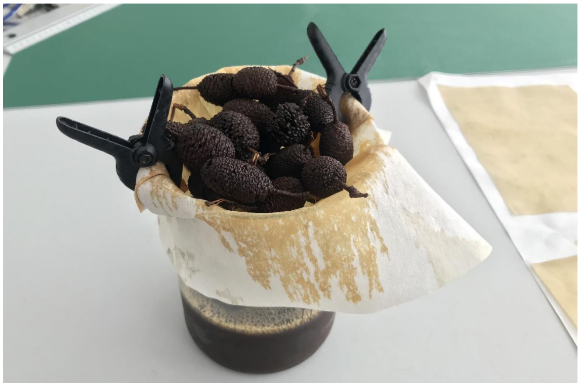
Figure 129. Preparation of the dye for toning paper from yasha cones, straining the solution through an unwoven textile fabric.
