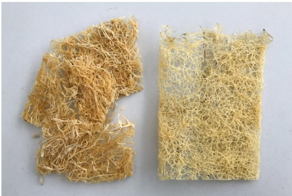
Figure 77. Funori (left), mafunori (right). Unlike funori , mafunori dissolves at room temperature, which makes it more reversible. It can be removed from the object at room temperature without being heated.
