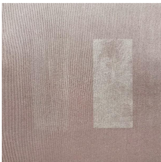
Figure 155. Surrogates with a tear along the warp direction mended with: a) paper patch; b) textile patch using adhesive Klucel G, dark background.
