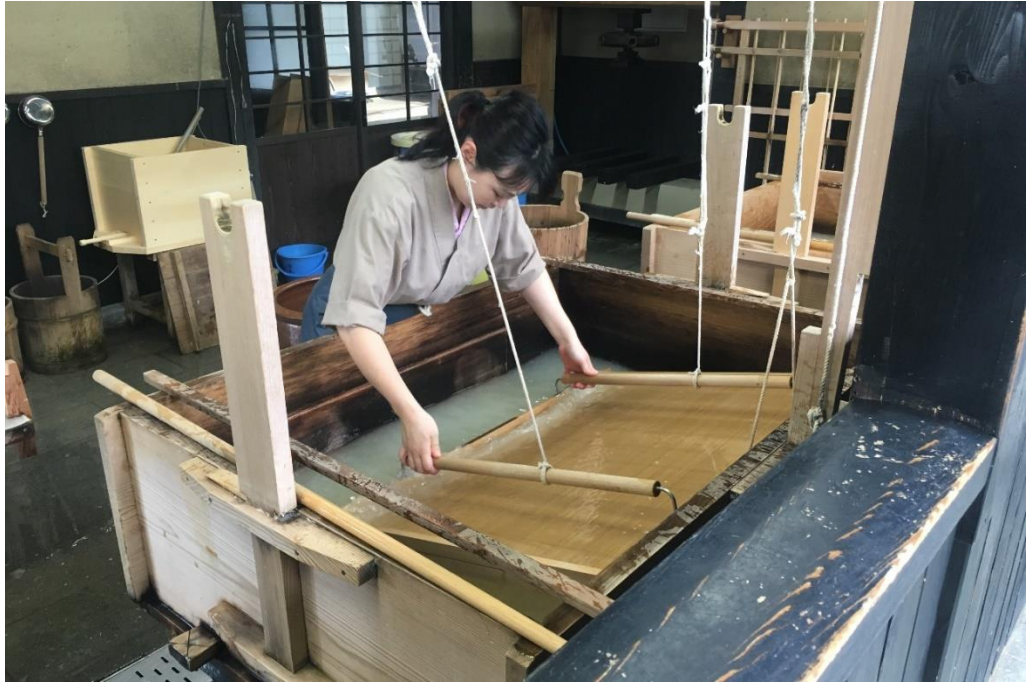
Figure 72. Process of forming sheets of paper using paper pulp, Japanese method.
