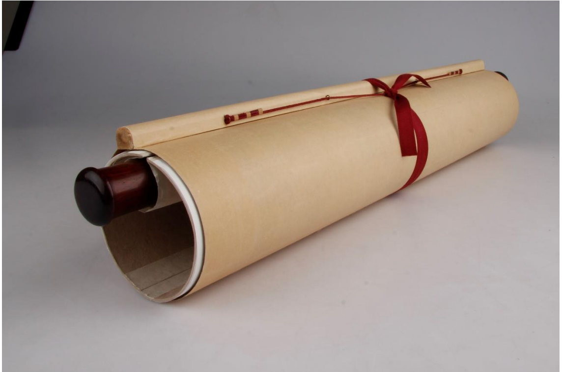
Figure 92. Futomaki roller made to reduce the possibility of creases and cracks appearing.
