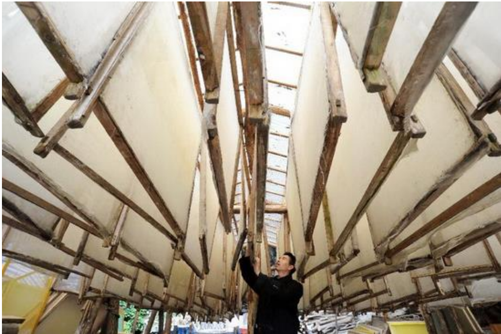
Figure 75. Process of drying paper, Chinese method. 63
