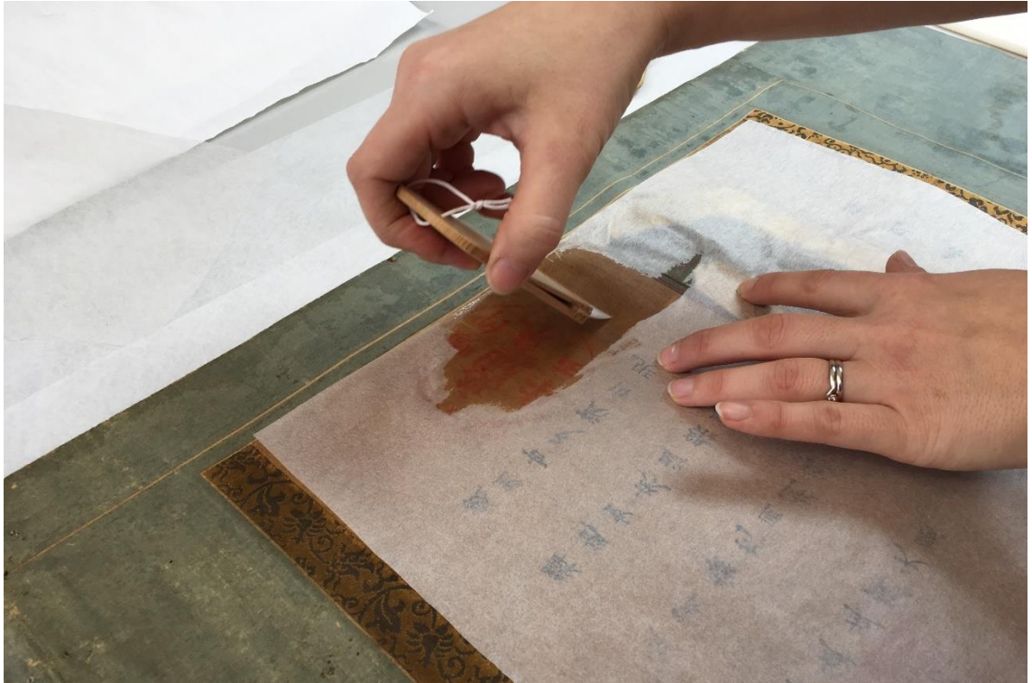
Figure 116. Facing using rayon paper, application of the first rayon paper layer on the painted part of the scroll.
