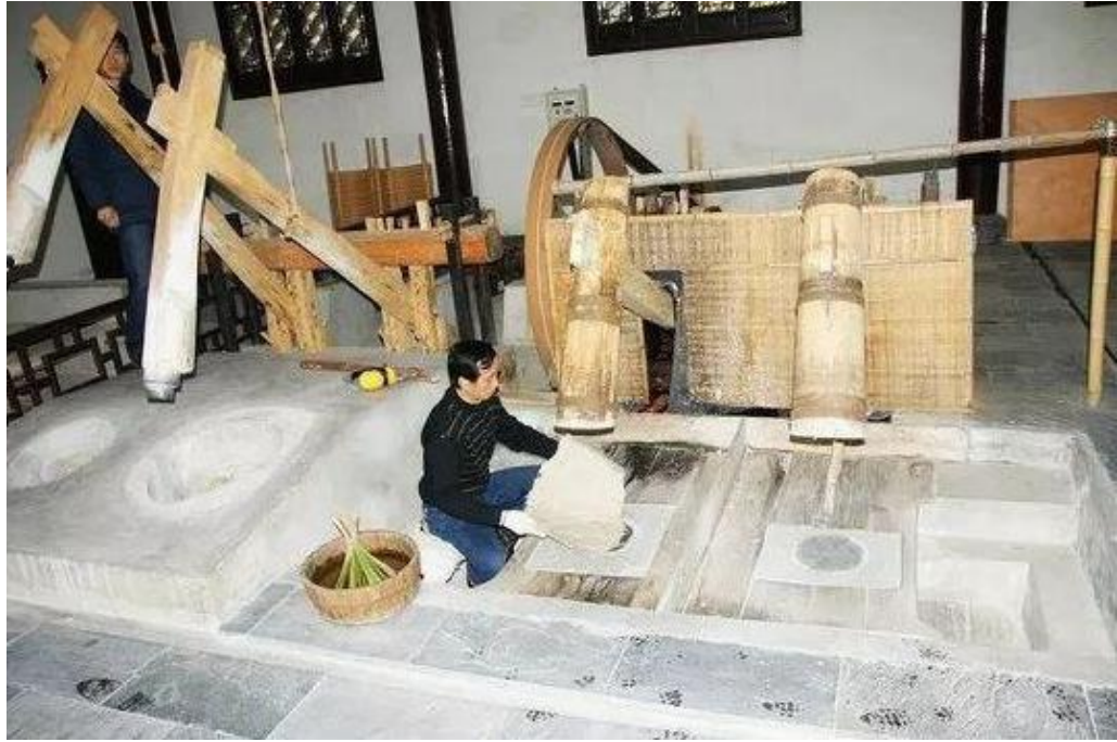
Figure 70. Chinese method of pounding the bast. 60
