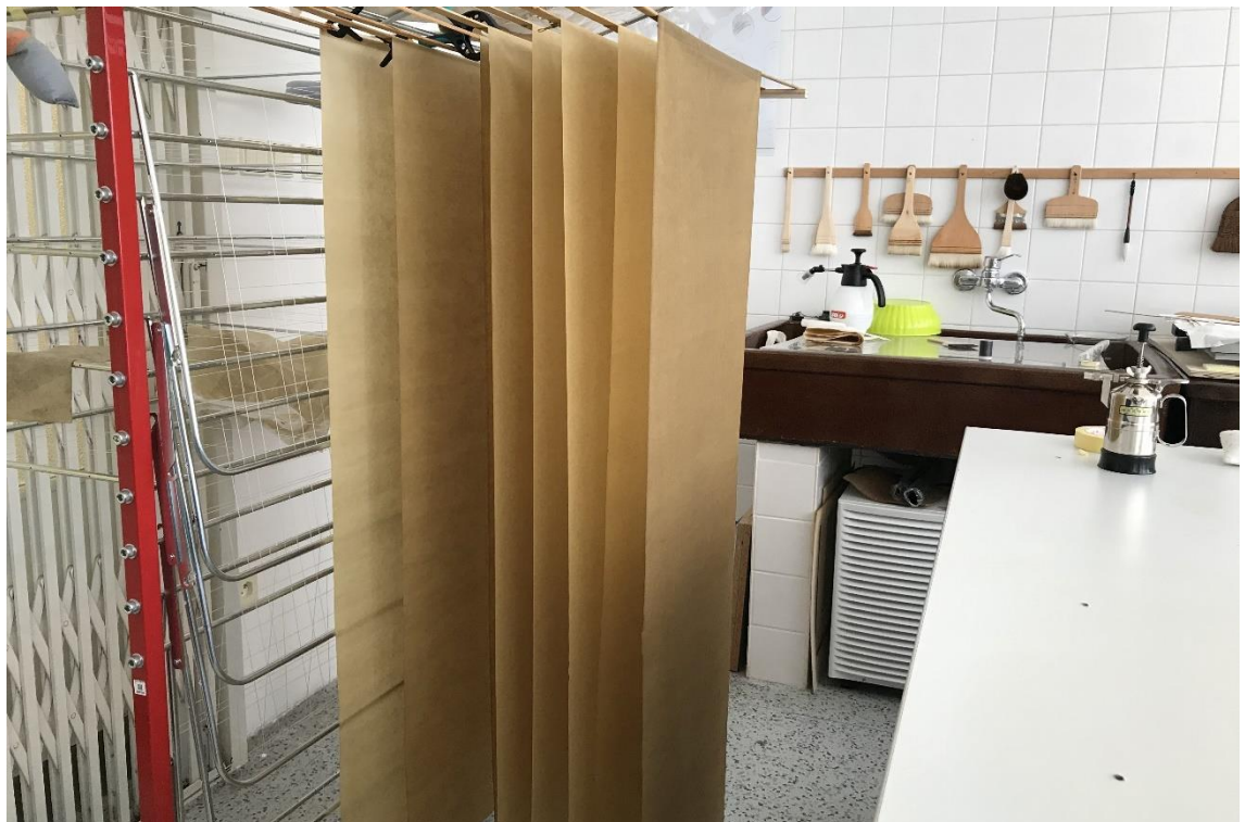
Figure 133. Preparation of the dye for toning paper from yasha cones, drying toned papers.
