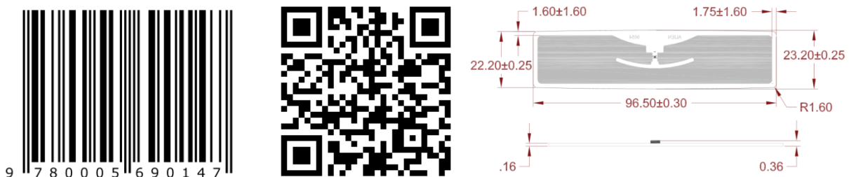
Fig. 1: EAN-13 code, QR code and RFID UHF tag ALN-9654 “G” Inlay used in the experimental measurements
