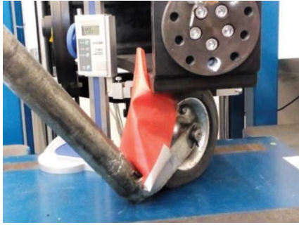
Fig. 11 Deformation of the support wheels on the static adhesor
