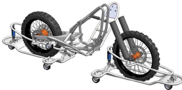
Fig. 13 Mechanical part of the SkidMotorbike system
