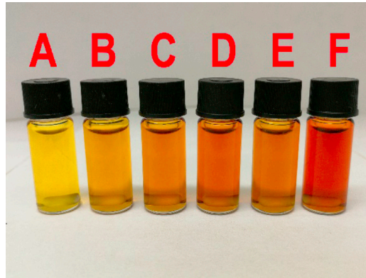
Fig. 1. Prepared \text{Ge}_{20}\text{Sb}_5\text{S}_{75} ChG solutions. A: 0.015, B: 0.03, C: 0.045, D: 0.06, E: 0.075, F: 0.09 g/ml BA.
