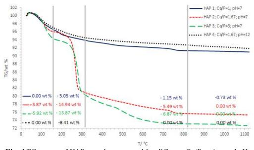
Fig. 4 TG curves of HAP samples prepared for different Ca/P ratios and pH.
