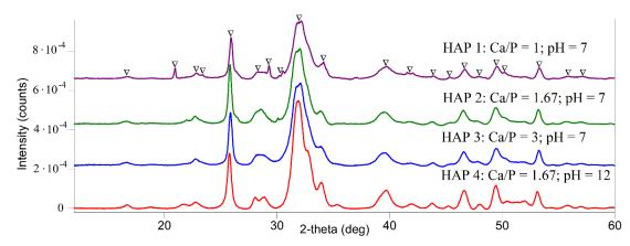
Fig. 1 Diffractogram of crystal system of hydroxyapatite.
