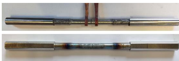
199 200 Figure 6. Heating the notched area of the round bar samples.
