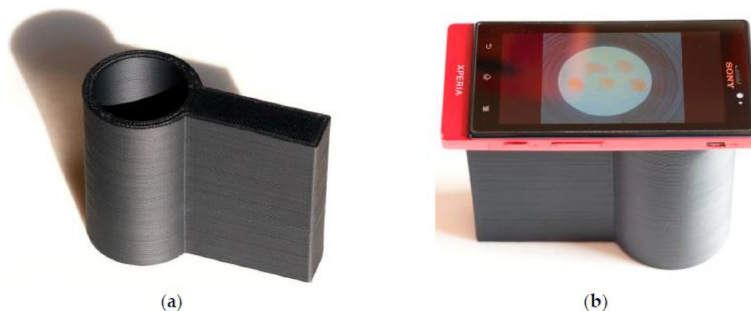
Figure 1. Tube-shaped holder (a) prepared using 3D-printing technology, and the final settings for photography (b).
