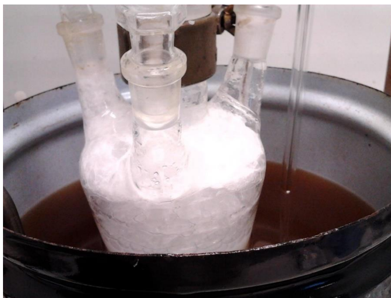
Figure 11: Bubbles formation during the reaction of \text{Zn(OH)}_2 with peroxide
