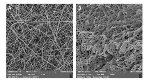
**Fig. 1** Scanning electron microscope image of chitosan nanofibers before (A) and after (B) hydratation, magnification 5,000 x. TESCAN VEGA3.
