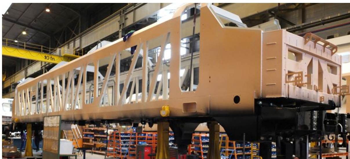
Obr. 29: Skříň lokomotivy Stadler UKLight (Class 68). Autor: Railway Gazette [33].
