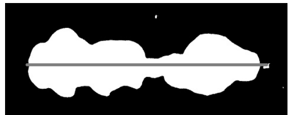
Fig. 5. White area is the area of delamination, gray is the area of the scribe.
