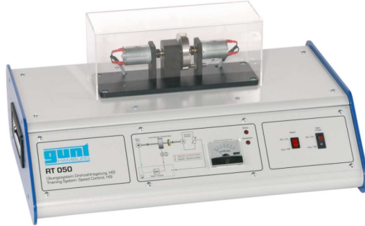
Fig. 2. GUNT RT 050 – speed control laboratory system
