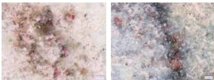
Figure 13 Layers of deposits and corrosion products in drops of uric acid + sodium nitrate and applied (Belgian) bird droppings after 4 weeks' exposure – eroded surface with red crystals. Photo: Kristen Balogh
