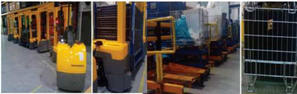
Fig. 1. Train T1 with the gantry wagons left and train T2 with transport basket. Source: authors
