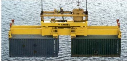
Fig. 1. Twin-lift spreader for two 20-foot containers. Source: www.vdlcontainersystemen.com
