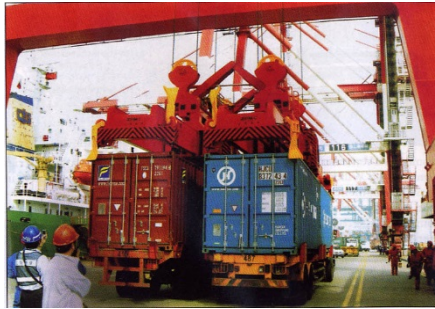
Fig. 2. Tandem spreader for two 40-foot containers. Source: www.dpworld.ae
