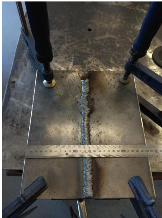
Figure 7.3 Welding of Strenx 700MC plates with clamping apparatus
