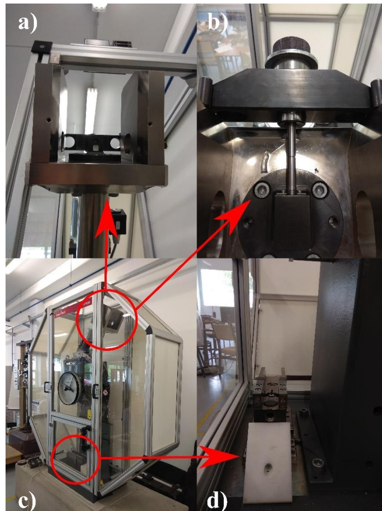
Figure 7.19 a) Pendulum hammer, b) Screwed specimen between tail block and tup, c) General view of Zwick/Roell RKP 450 pendulum impact tester and d) Anvil
