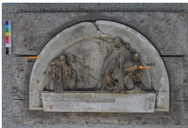
Fig. 2: Sample vz.1/8608 and vz.2/8609 B taken from the relief. Vz.1 was taken from the frame (rám), vz.2 was taken from the inner part of the relief from one of the figure. Author: K. Teturová.
