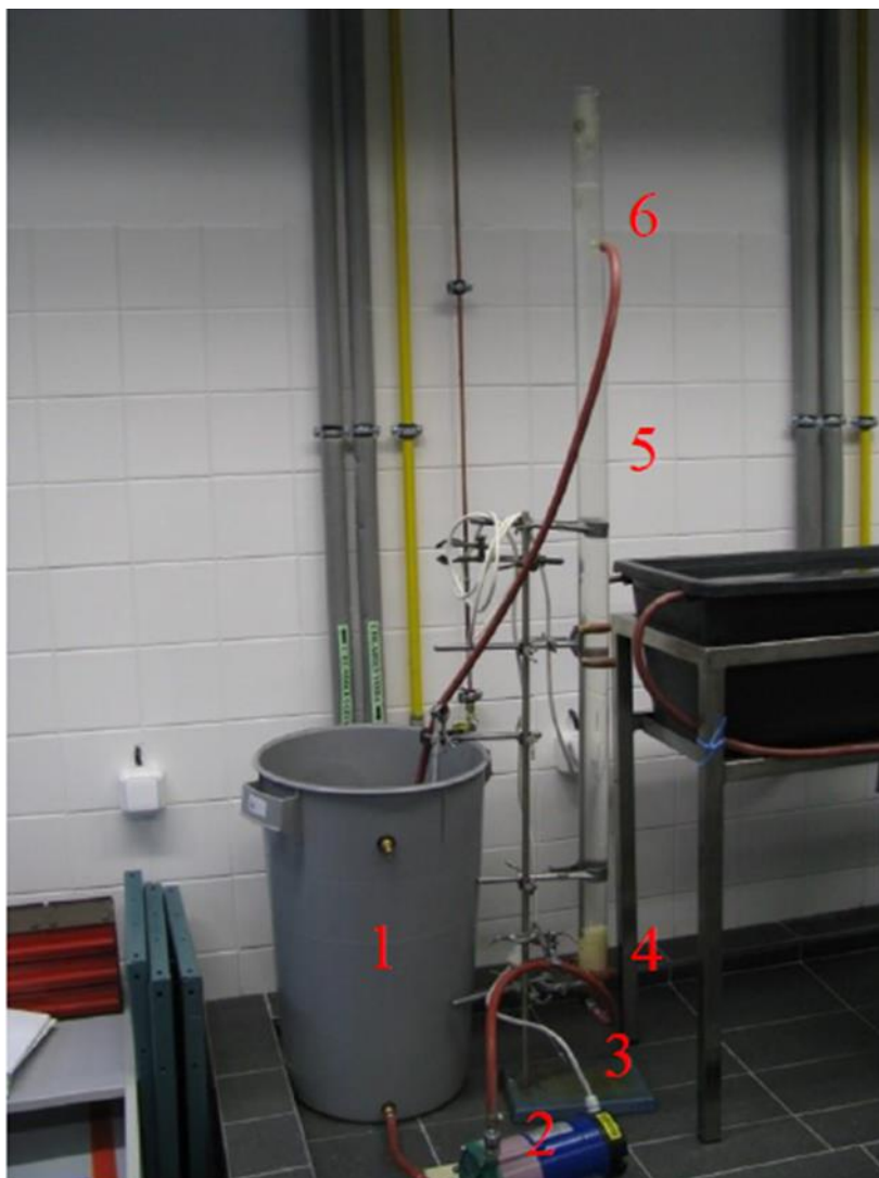
Fig. 2 Fluidized bed reactor: 1 – reservoir with model wastewater, 2 – pump, 3 – inflow of model wastewater, 4 – fluidized biopellets, 5 – column, 6 – overflow of wastewater back into the reservoir
