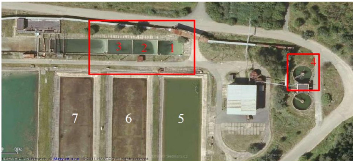
Fig. 4 The Pustý area with a cascade of three lagoons used for pilot experiments (1, 2, 3 – lagoons, 4 – circular tank for preparation of model wastewater, 5, 6, 7 – large lagoons used for real wastewater treatment)
