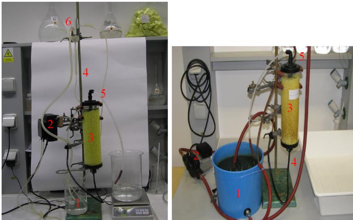
Fig. 3 Sulphur denitrifier apparatus (flow mode on the left, circulation mode on the right): 1 – reservoir with model wastewater, 2 – pump, 3 – column packed with sulphur granules, 4 – inflow of model wastewater, 5 – outflow from column, 6 – overflow of wastewater
