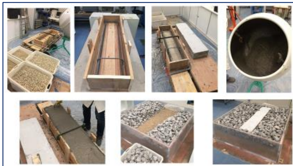
Figure 6.36. Preparation of Sleepers and placing them in the tank
