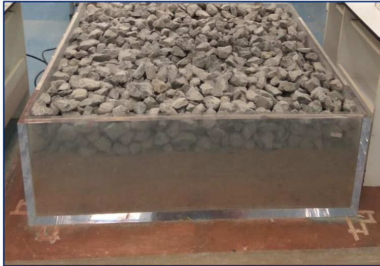
Figure 6.35. The fouled condition of ballast in the tank at the beginning of the laboratory experiments
