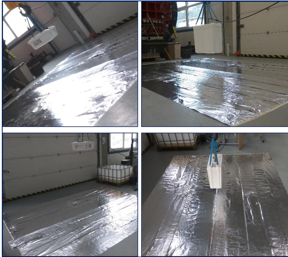
Figure 6.1. Pictures during surveys for GPR performance compliance tests: left side pictures: ground-coupled antenna (400/900MHz), right side pictures: air-coupled antenna (2GHz)
