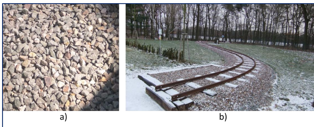
Figure 6.8. a) Fine-sized granite ballast stones used during the experiments, b) exactly the same type of granite aggregates used for the test track
