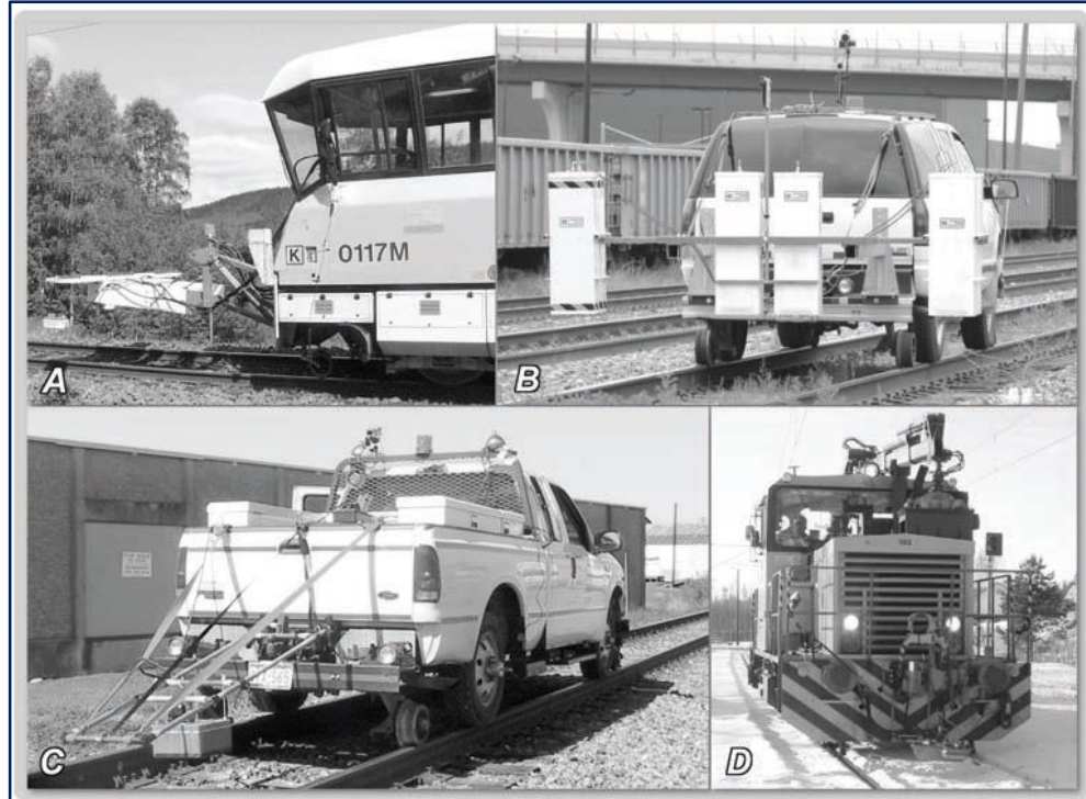
Figure 4.2. Different GPR sets used in Railways [56]: a) Swedish Mala ground-coupled antenna (photo by Mala Geoscience), b) multichannel GSSI air-coupled system (from Olhoeft et al. [81]), c) GSSI 400MHz ground-coupled antenna and d) Radar Team Sweden 350MHz 1.2GHz Sub-Echo HBD antennas (photo Mika Silvast)
