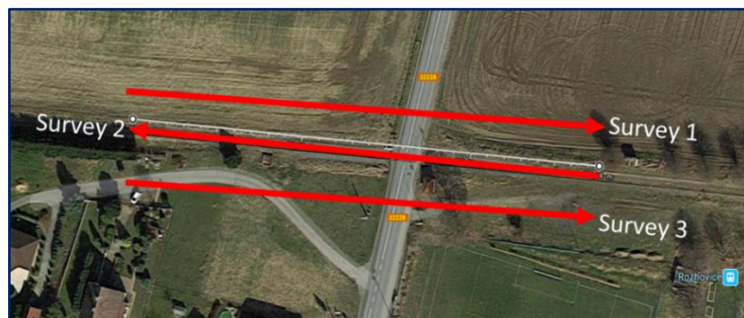
Figure 6.22. Advancing directions of the GPR surveys held with GPR set of University of Pardubice
