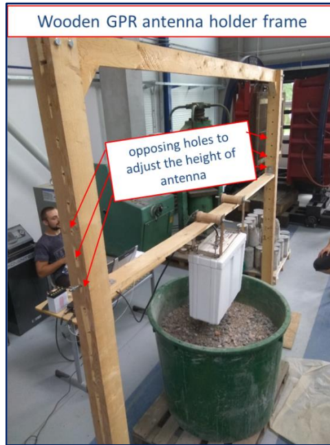
Figure 6.3. Wooden GPR antenna holder frame
