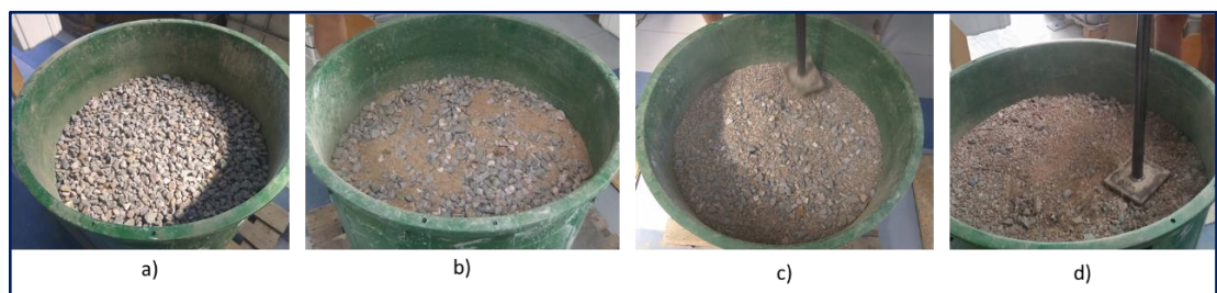
Figure 6.5. Configurations of a) clean b) sand-fouled c) fine gravel-fouled d) mixture-fouled finer granite ballast
