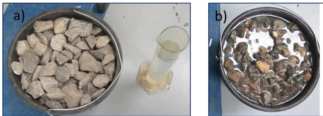
Figure 6.10. Calculation process of air voids content by volume for both ballast types a) coarse sized-granite ballast b) fine-sized granite ballast
