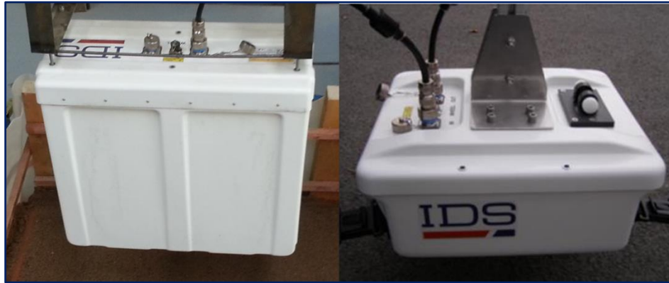
Figure 5.2 IDS antennas: left picture air-coupled 2GHz horn antenna, right picture ground-coupled TR dual frequency antenna (400/900MHz)
