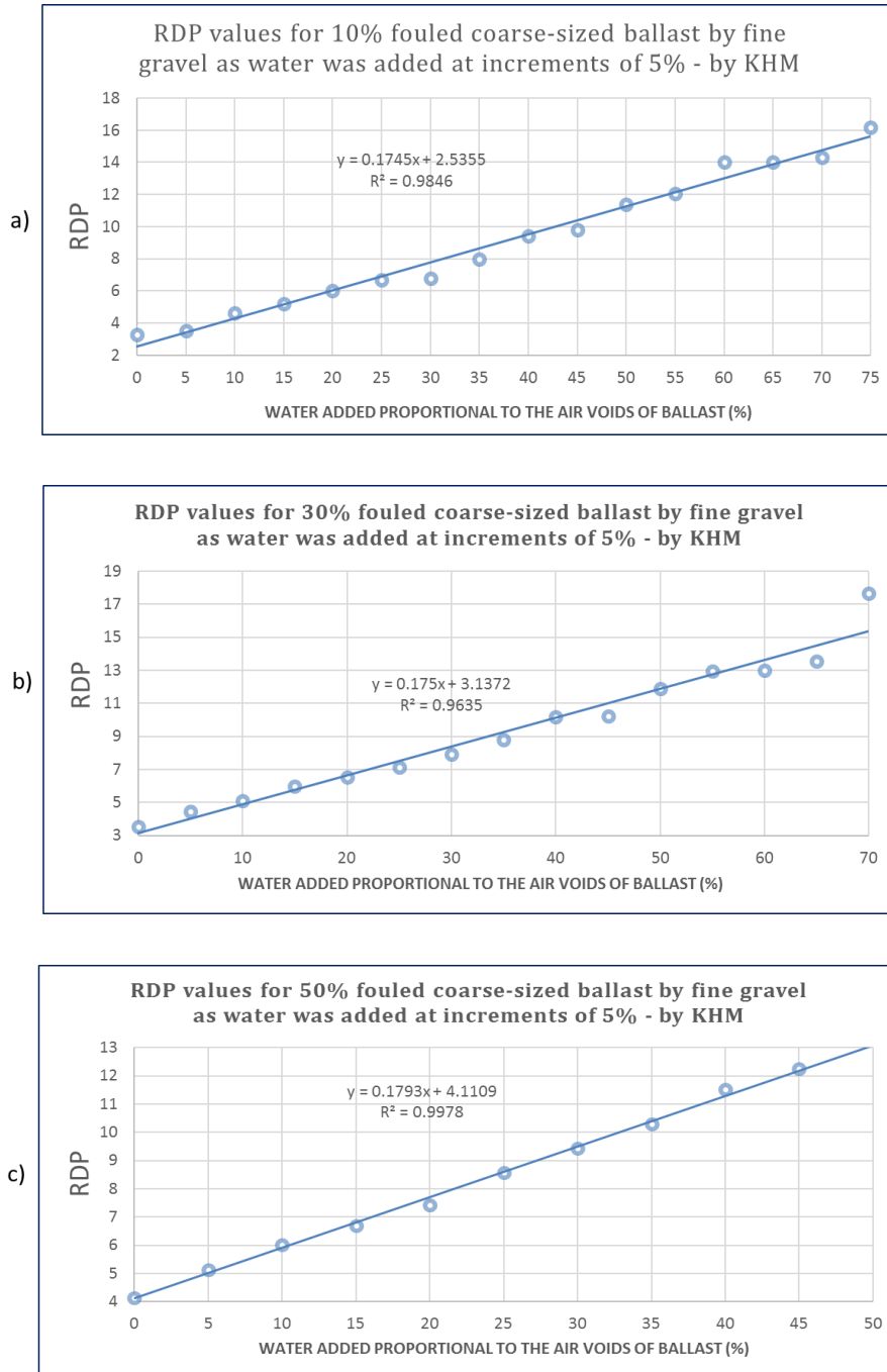
Figure 7.10. RDP values for fouled coarse sized granite ballast under gradual water addition at specific levels of fine gravel fouling a) 10%, b) 30%, c) 50% fine gravel fouled ballast
