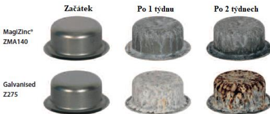
Obr. 21 - Test protikorozi odolnosti v solné mlze [17]
