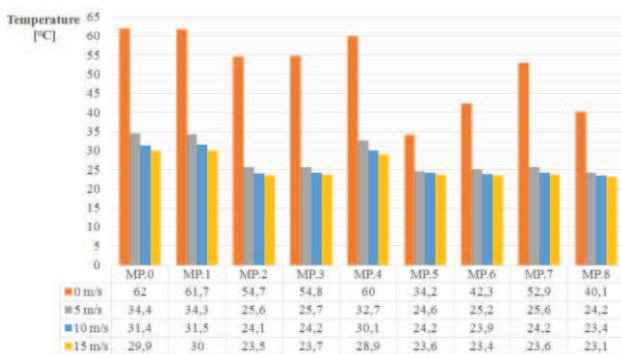
Fig. 17. Comparison of temperatures in points 1-8 based on simulation for air-flow 0; 5; 10 and 15 \text{ m}\cdot\text{s}^{-1} .
