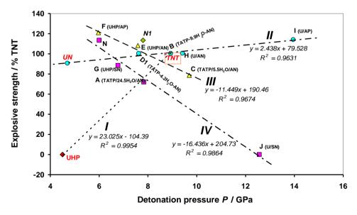
Fig. 1. Mutual relationship between experimental relative explosive strength and calculated detonation pressure of the studied mixtures
