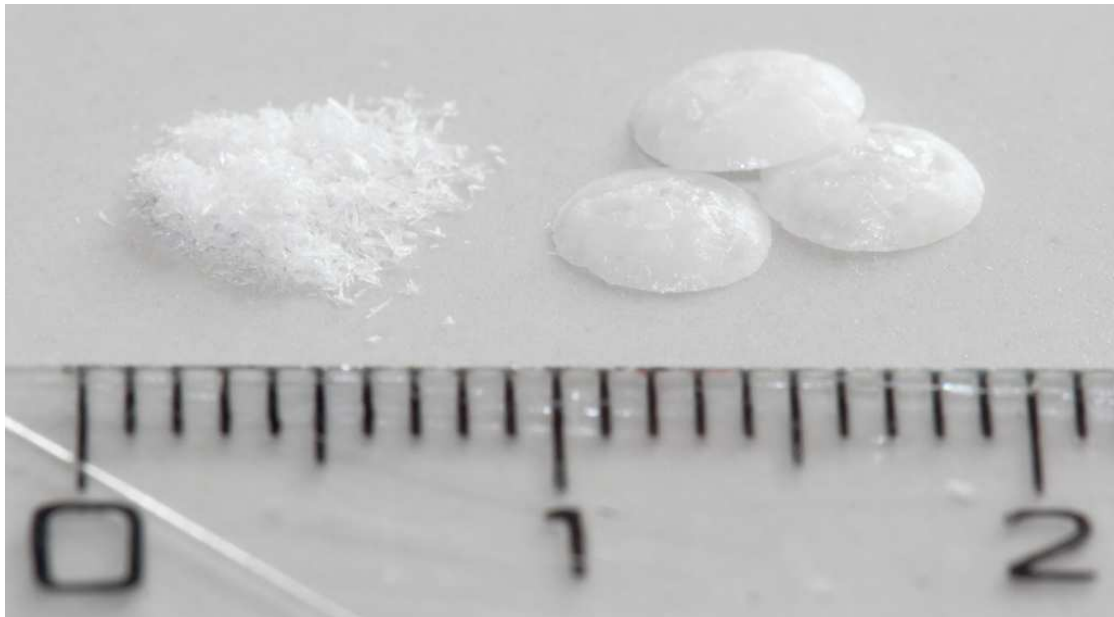
Figure 1. Shape and size of crystalline ETN (left) and melt cast ETN pellets (right). The fine scale division is in millimeters.
