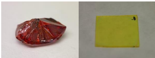
Figure 2: The As 30 S 70 source bulk glass (left) and as-prepared spin-coated thin film (right).
