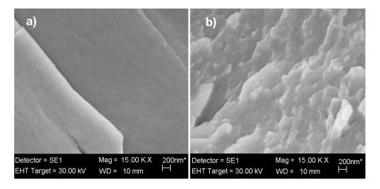
Fig. 6 Cryo-fracture surface of the coating film based on the acrylic binder Veropal D
