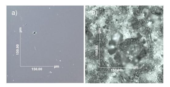
Fig. 5 Cryo-fracture surface of the coating film based on the acrylic binder Synthalat A 125 HS a) without the addition of nanogels, b) containing 40 wt. % of nanogels
