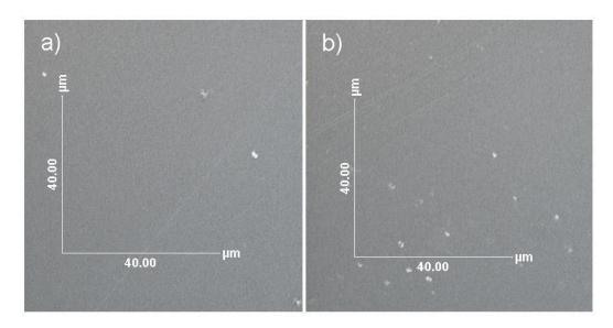
Fig. 4 Appearance of coatings based on the acrylic binder Veropal D 709 containing a) 0 wt. % of nanogels, b) 40 wt. % of nanogels
