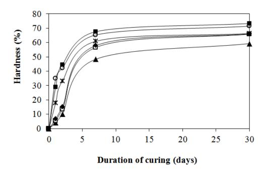
Fig. 8 Effect of time and nanogel content in the acrylic binder Veropal D 709 on the pendulum hardness of coatings. The content of nanogels: 0 wt. % (♠), 10 wt. % (□), 20 wt. % (♦), 30 wt. % (\*), 40 wt. % (■), 50 wt. % (⋄) is related to the total amount of solids in the coating
