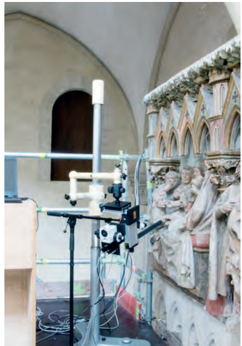
Fig. 10 (right) Measuring head of the mobile Raman microspectrometer in use at the relief of Naumburg west rood screen (Photo Jacqueline Menzgel)
