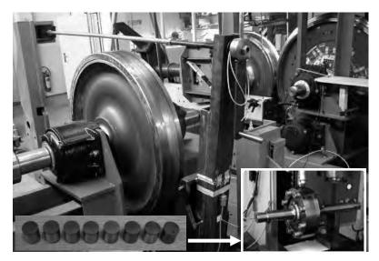
Figure 1 Rolling-contact fatigue testing equipment, detail on holder for set of tested samples
