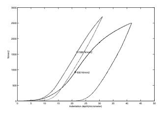
Figure 4 Finding Comparative yield stress CYS [N/mm<sup>2</sup>] by using cylindrical indenter (red line explosive hardening, blue line without exp. hardening)
