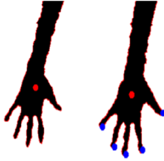
Figure 3.5: Result of k-curvature fingertip detection
