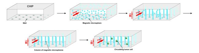
The Ephesia system. Alligment of magnetic microspheres into columns inside the chip under magnetic field and capture of epithelial cells.
