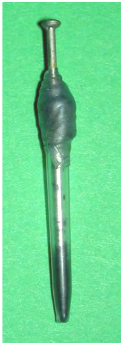
Fig. 1: Photograph of the carbon paste microelectrode (CP \mu\text{E} ), showing the plastic micropipette tip body, the carbon paste filling at the bottom of the tip and the stainless steel nail current collector immersed into the wider end of the tip and fixed with parafilm.
