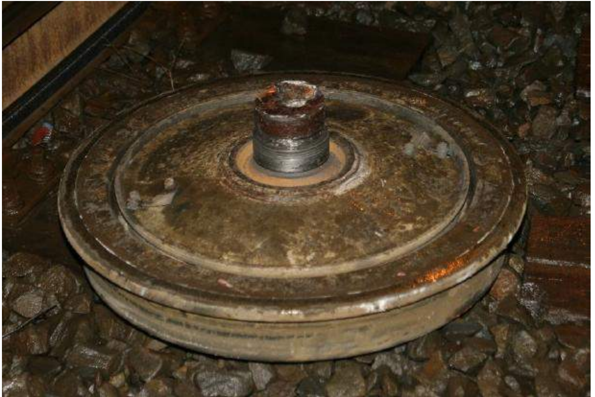
Figure 9 - A wheel of a tram from Ostrava with a part of broken axle [13]
