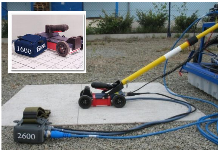
Fig. 1 Georadar equipment – hand cart (model 615)
