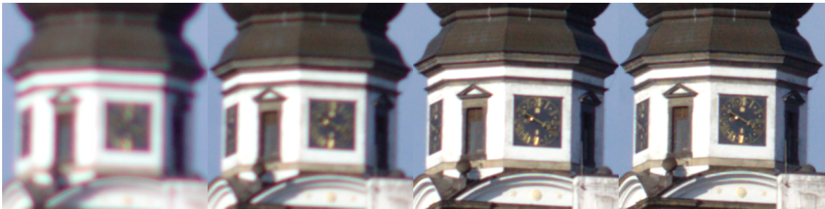
Obr. 6.9: Vliv clony na ostrost - Canon EOS 5D Mark II, (f 1,4; f 2,8; f 5,6; f 11), 400x400 ob
