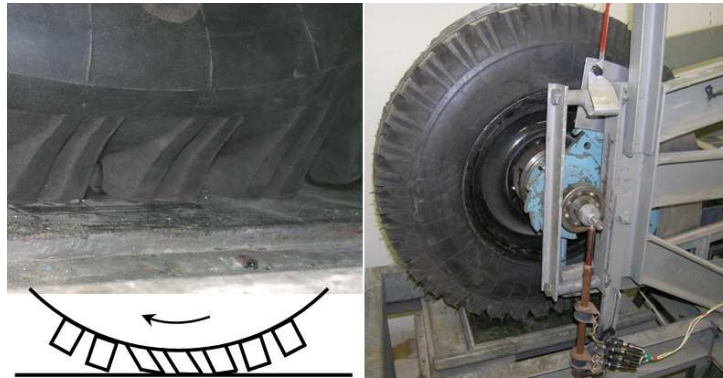
Figure 3 Statical adhesion with contact area detail
